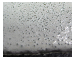
Material after heating with ideal 60% glass bead embedment for optimal performance
